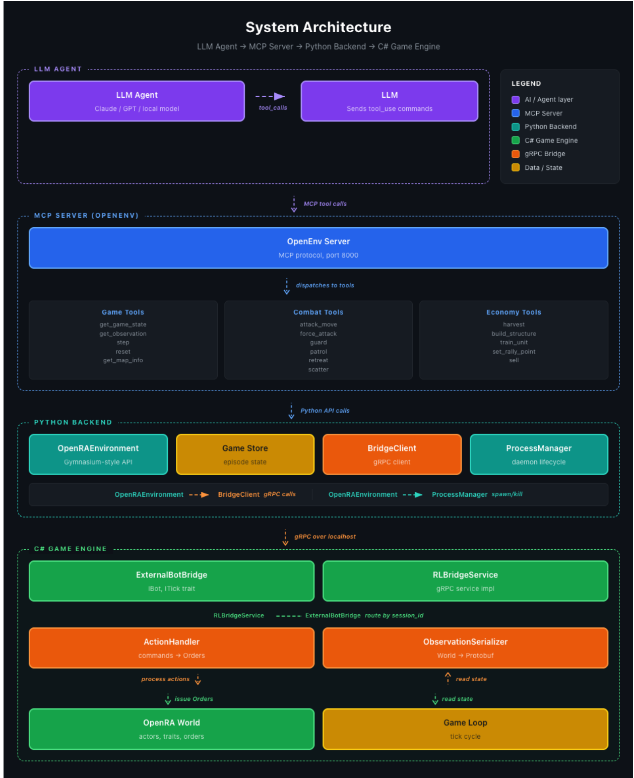
Figure 1: System architecture of OpenRA-RL. The platform consists of three interconnected layers: LLM agents interact through the Model Context Protocol (MCP) server, which communicates with a Python backend via FastAPI, and the Python backend connects to the C# game engine through a gRPC bridge. This modular design decouples agent computation from game execution, supporting diverse agent paradigms from scripted bots to LLM-based reasoners.
