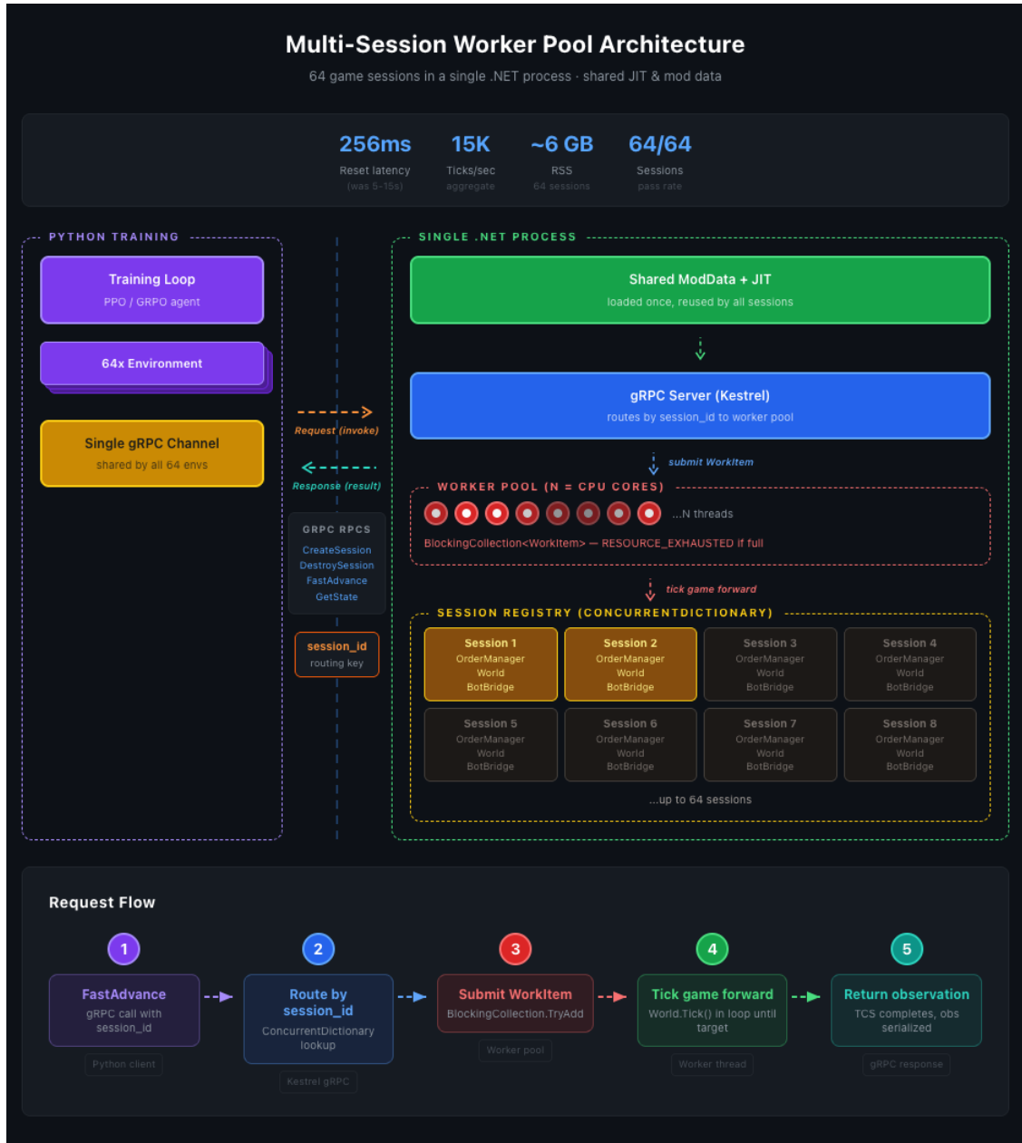
Figure 3: Multi-session worker pool architecture (v2). Up to 64 concurrent game sessions run within a single .NET process, sharing immutable ModData to eliminate redundant memory usage. Game ticks are processed by a dedicated worker thread pool separate from gRPC request handlers, preventing resource contention. Each session is protected by a per-session semaphore for safe parallel execution.
