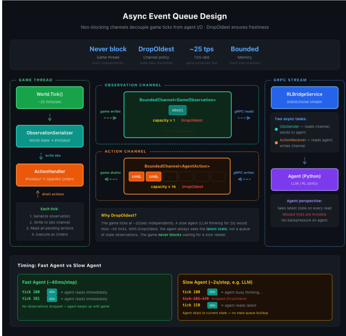
Figure 2: Asynchronous event queue design with bounded, non-blocking channels. The observation channel (capacity=1, DropOldest) ensures agents always receive the most recent game state, while the action channel (capacity=16) buffers agent commands. This asymmetric design decouples game ticks from agent inference time, allowing both fast scripted bots (~40ms) and slow LLM agents (~2s) to interact with the same 25Hz game engine.
